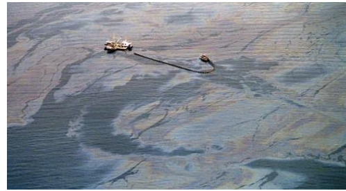
Figure 4: "Attempt to skim oil from the surface of the waters of Prince William Sound"
